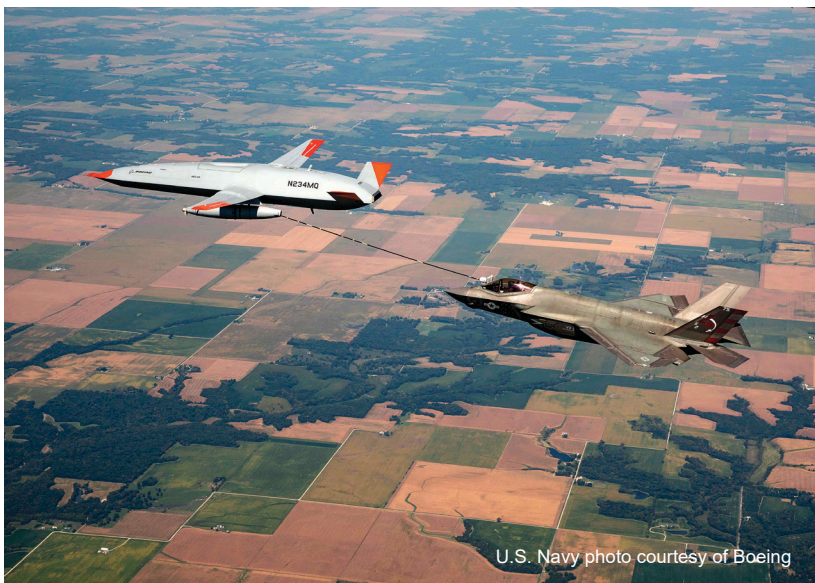
An unmanned Boeing MQ-25 T1 Stingray test aircraft, left, refuels a manned F-35 Lightning II. The MQ-25A Stingray will be the world's first operational carrier-based unmanned aircraft and provide critical aerial refueling and intelligence, surveillance and reconnaissance capabilities that greatly expand the global reach, operational flexibility and lethality of the carrier air wing and carrier strike group.
